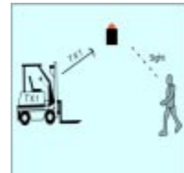
Fork Transmit to wall light for pedestrian vision
